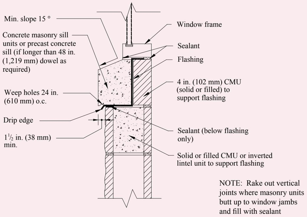
**Figure 6—Flashing Single Wythe Walls at Sills**
