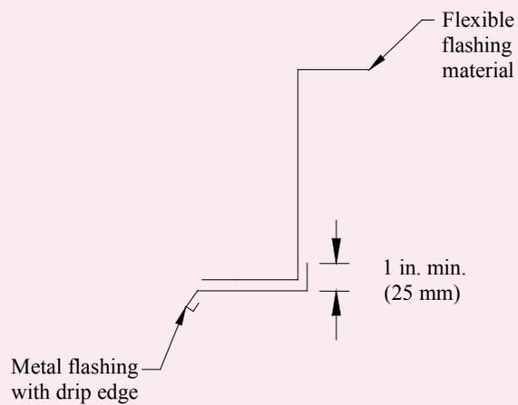
**Figure 5—Two-Piece Flashing Detail**
