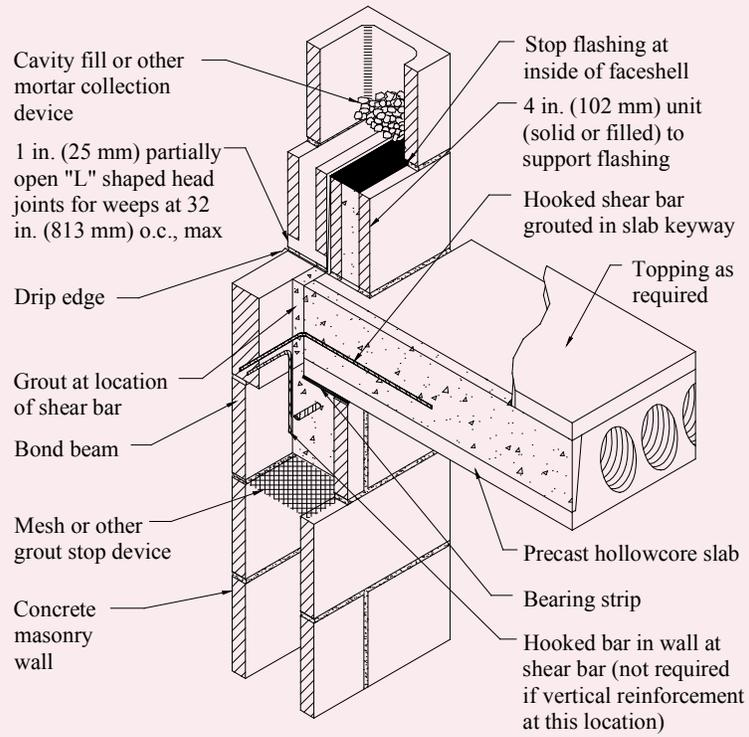
**Figure 4—Flashing Single Wythe Walls**
