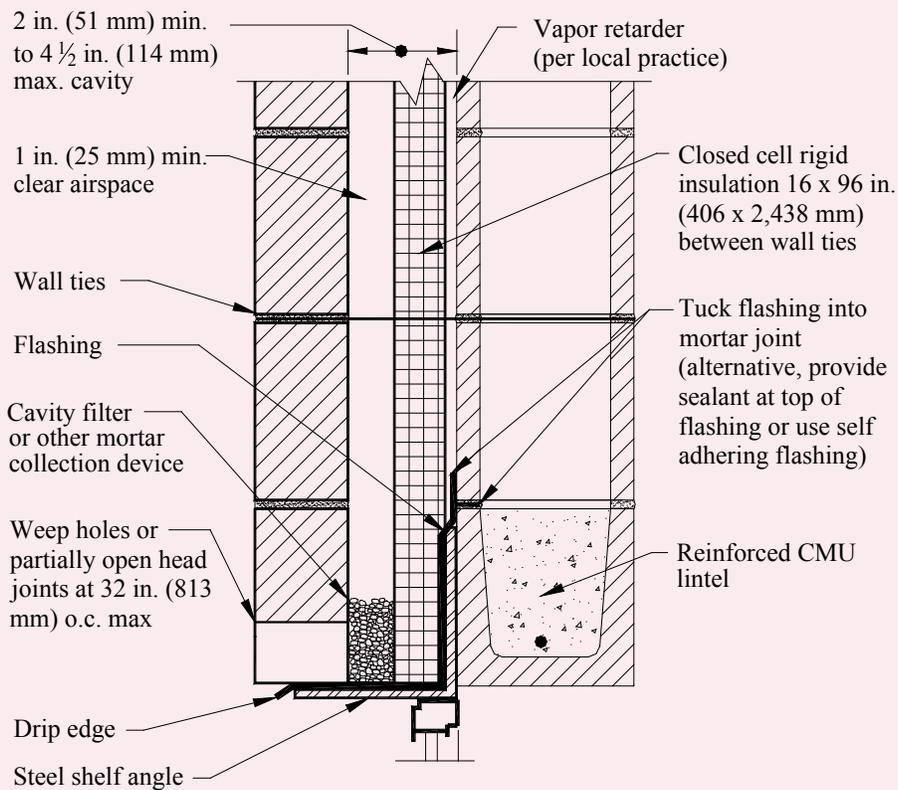
**Figure 2—Flashing Cavity Walls at Bond Beam Locations**
