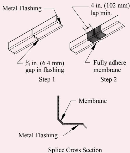
Figure 10—Splicing Metal Flashing
