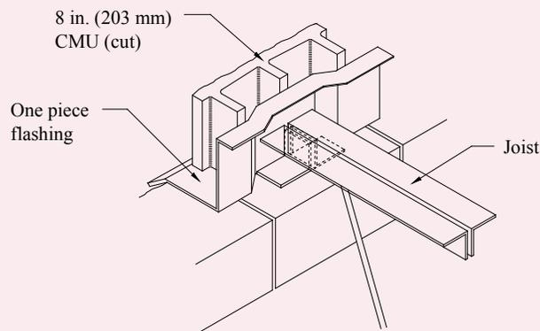
**Figure 8a—Isometric of Flashing Around End of Joist (ref. 5)**
