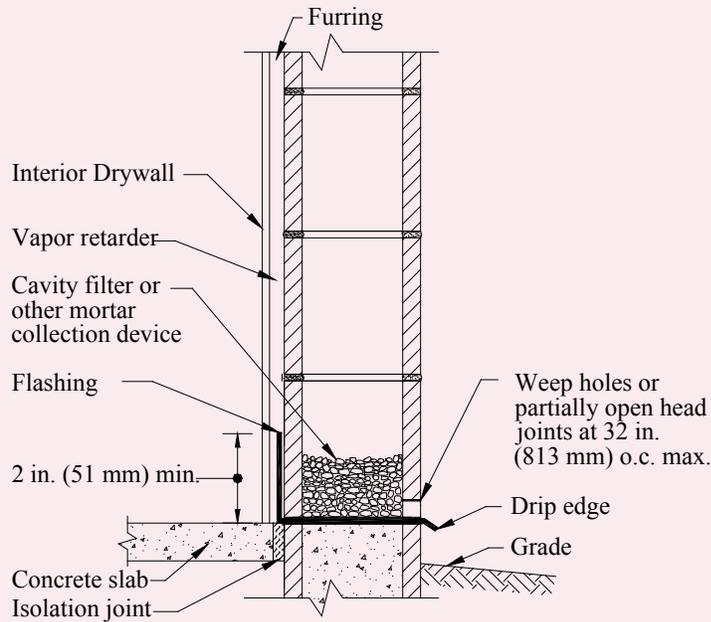
NOTE: The structural effect of through-wall flashing must be carefully evaluated.
