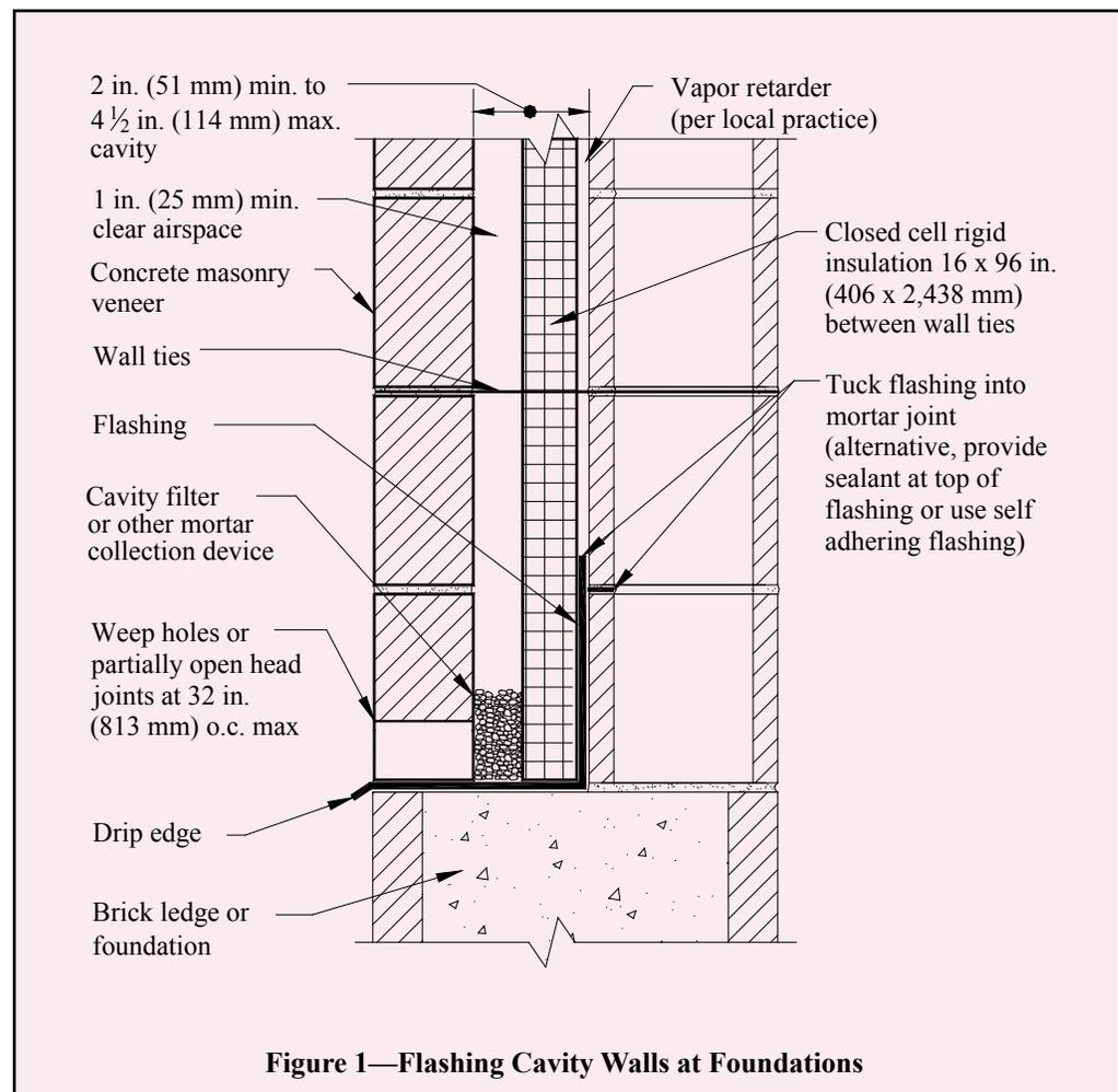
Figure 1—Flashing Cavity Walls at Foundations
