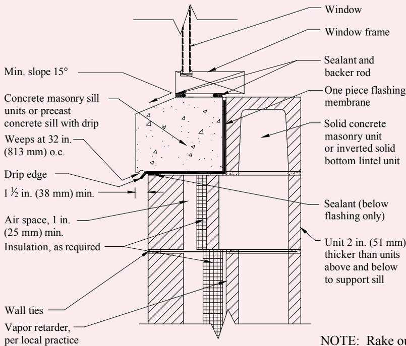
NOTE: Rake out vertical joints where masonry units butt up to window jambs and fill with sealant
