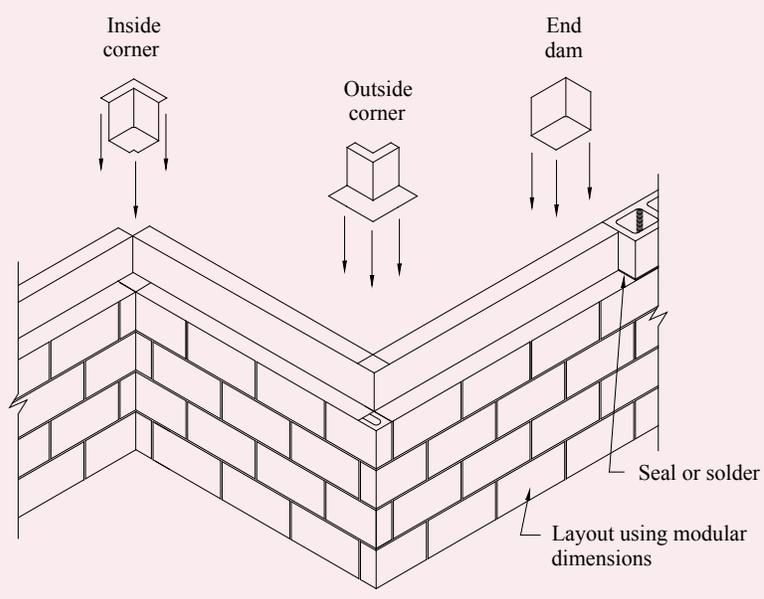
**Figure 7—Prefabricated Flashing Boots**
