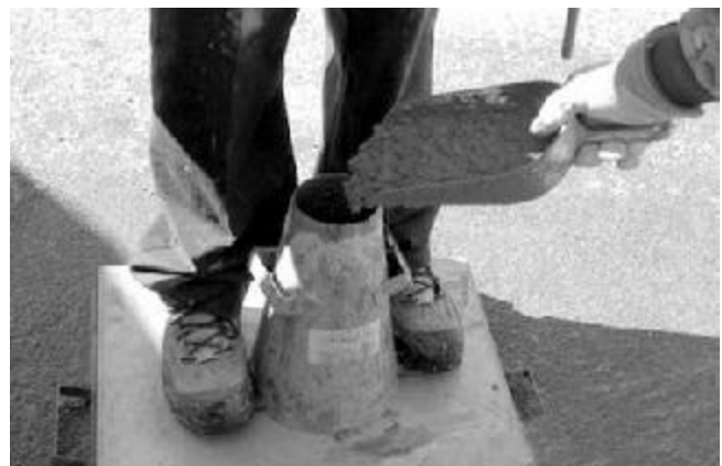
Figure 1—Filling the Slump Cone
