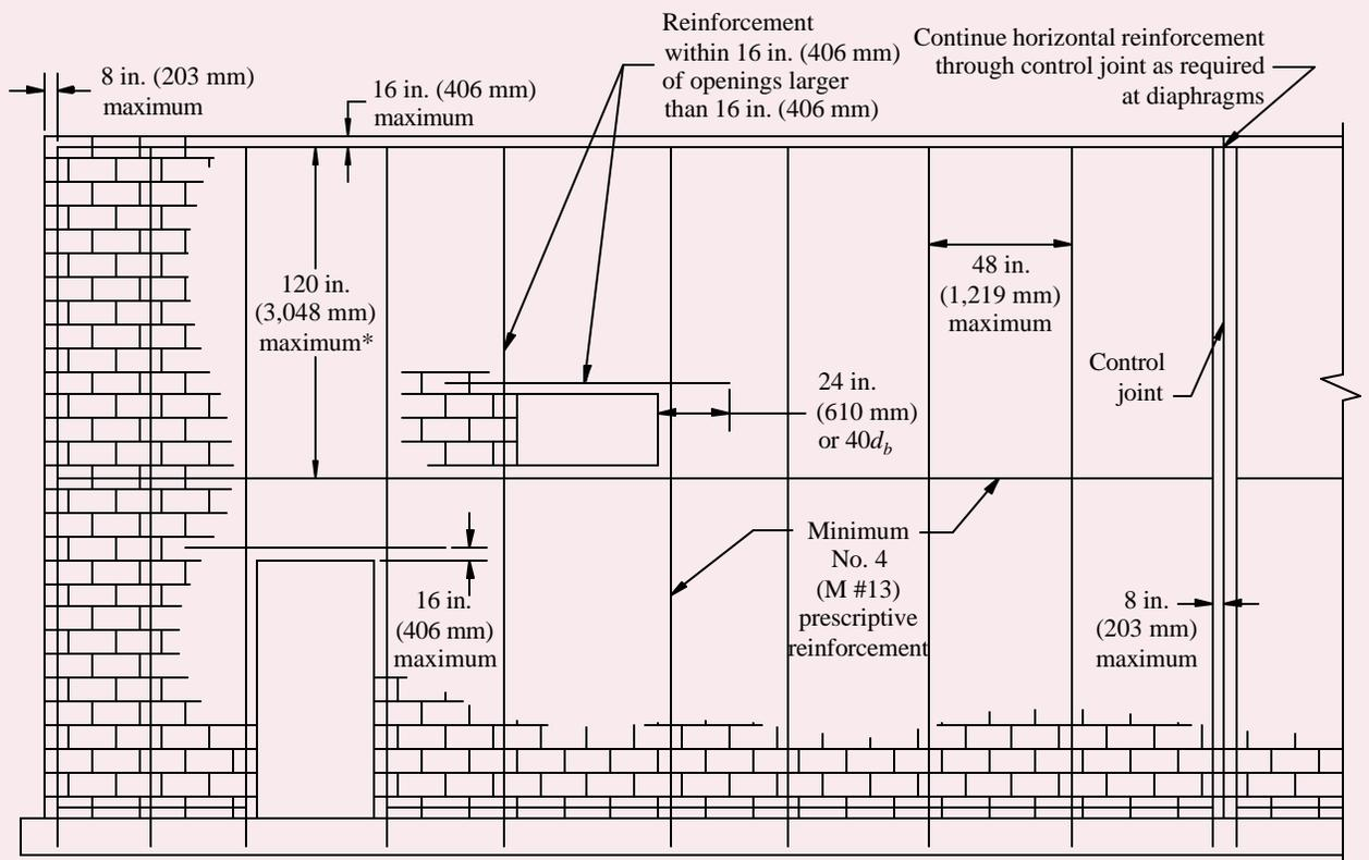
\*In lieu of bond beams with No. 4 bars (M #13) at 120 in. (3,048 mm) on center, provide two wires of wire size W1.7 (MW 11) joint reinforcement at 16 in. (406 mm) on center.
