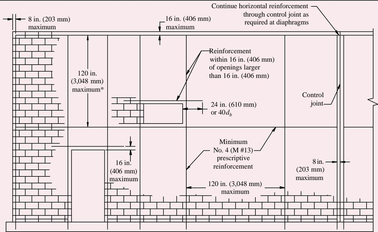
\*In lieu of bond beams with No. 4 bars (M #13) at 120 in. (3,048 mm) on center, provide two wires of wire size W1.7 (MW 11) joint reinforcement at 16 in. (406 mm) on center.
