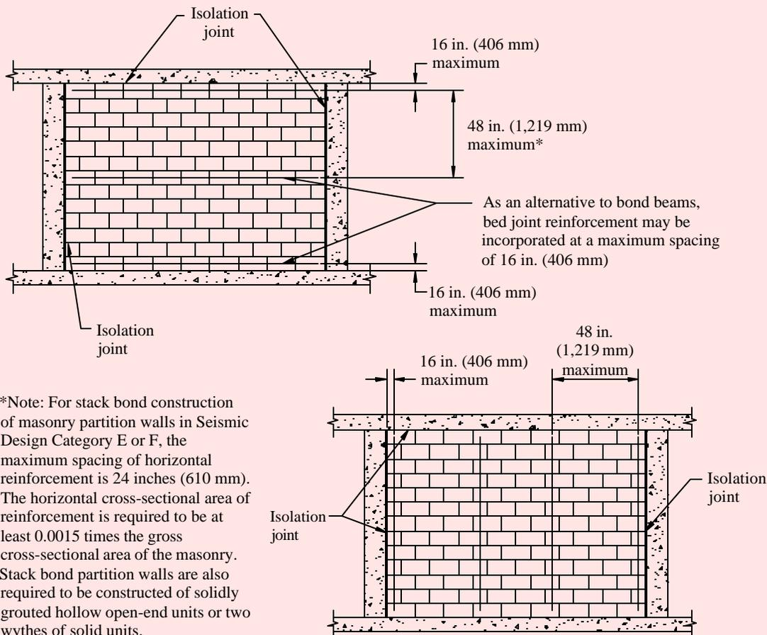
\*Note: For stack bond construction of masonry partition walls in Seismic Design Category E or F, the maximum spacing of horizontal reinforcement is 24 inches (610 mm). The horizontal cross-sectional area of reinforcement is required to be at least 0.0015 times the gross cross-sectional area of the masonry. Stack bond partition walls are also required to be constructed of solidly grouted hollow open-end units or two wythes of solid units.
