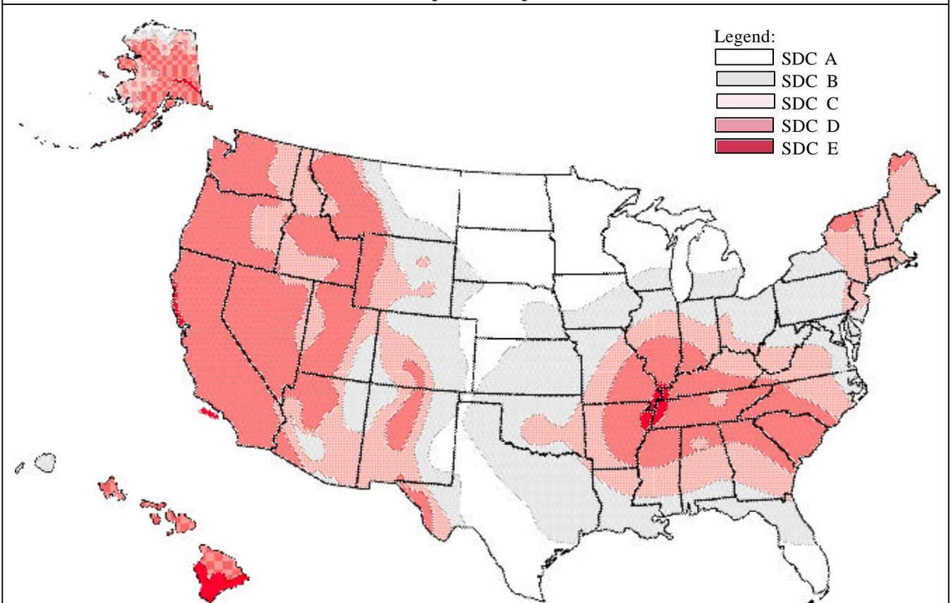
**Figure 2—Seismic Design Categories for Site Class D, Seismic Use Group I and II, for a 1-Second Spectral Response Acceleration**
