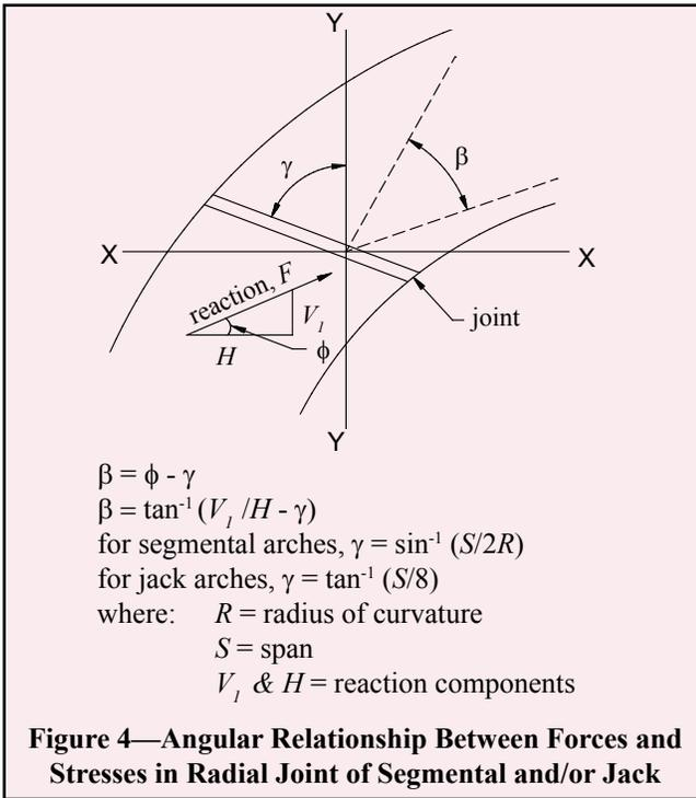
**Figure 4—Angular Relationship Between Forces and Stresses in Radial Joint of Segmental and/or Jack**
