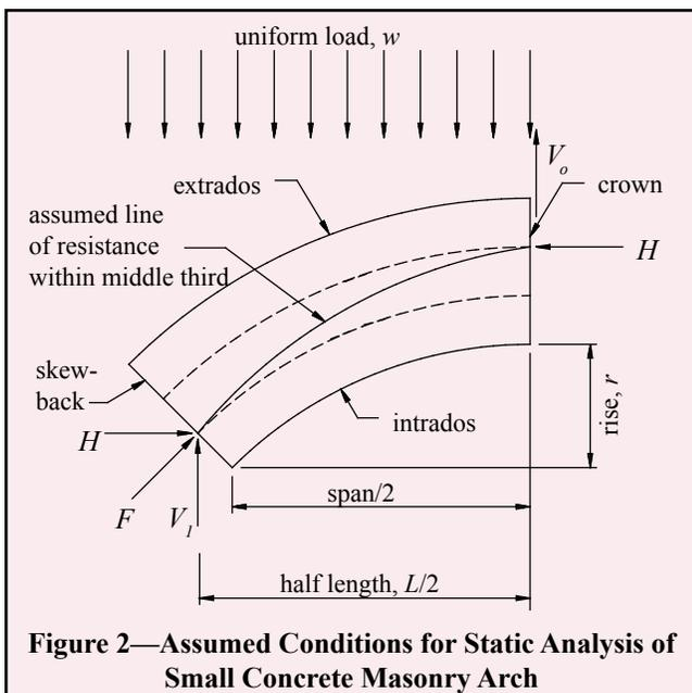
**Figure 2—Assumed Conditions for Static Analysis of Small Concrete Masonry Arch**
