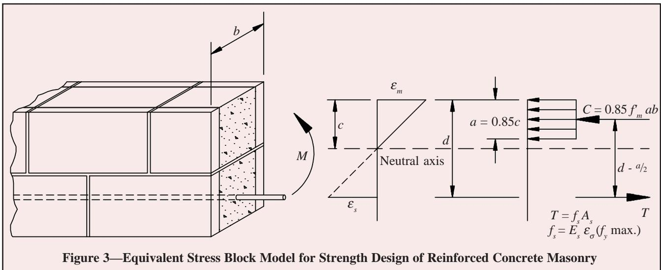
balanced strain conditions,  $\rho_{bal}$  (ref. 7). Balanced conditions occur when reinforcement reaches its specified yield strength at the same time that masonry reaches its maximum usable compressive strain of 0.003. This limit on reinforcement ensures the steel yields at strength level loads.
