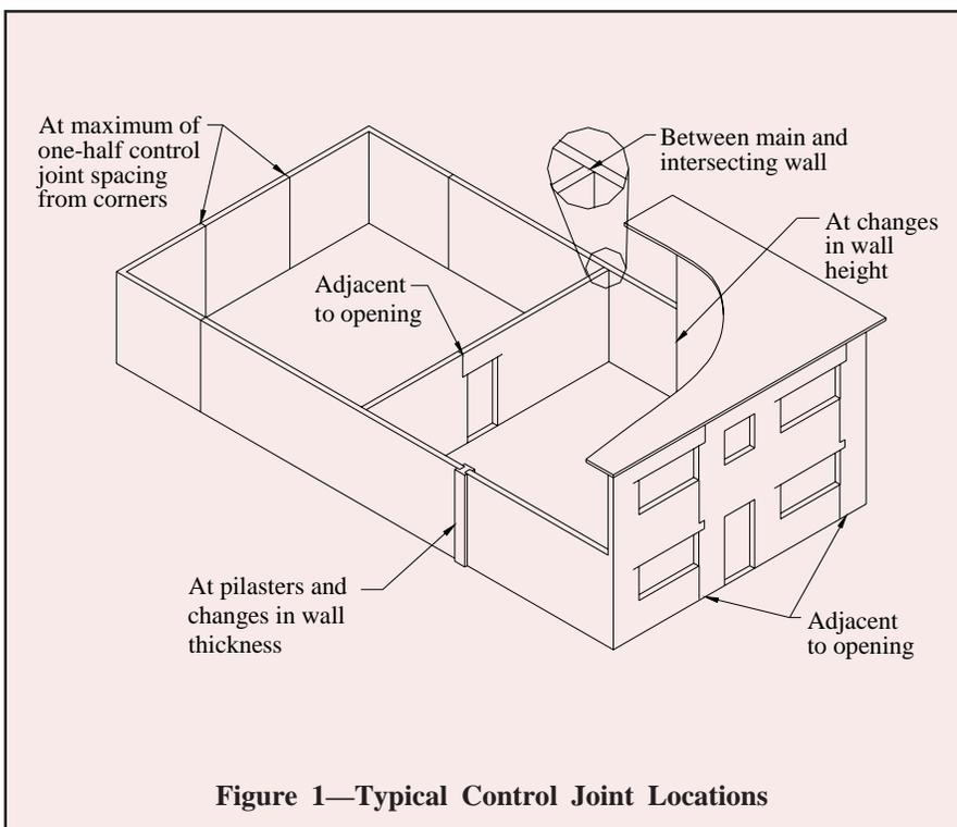
**Figure 1—Typical Control Joint Locations**
