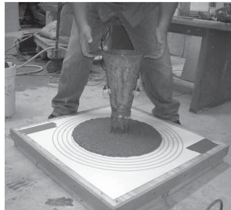
Figure 1—SCG Slump Flow Test
