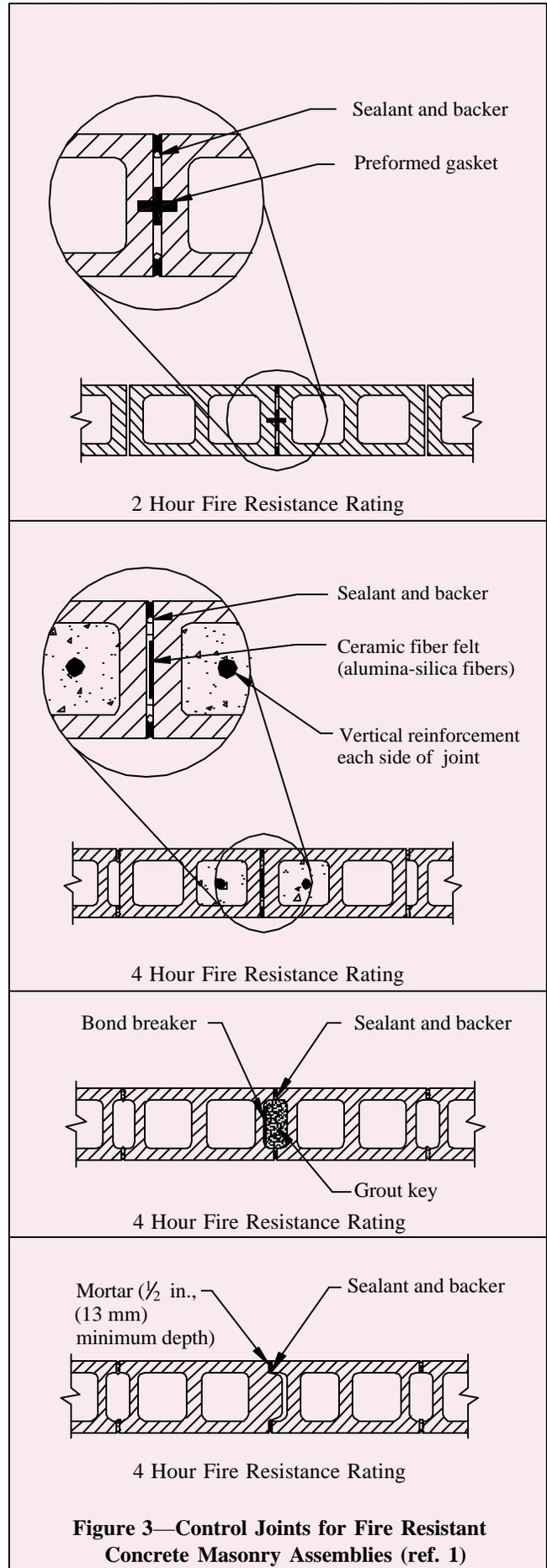
**Figure 3—Control Joints for Fire Resistant Concrete Masonry Assemblies (ref. 1)**
