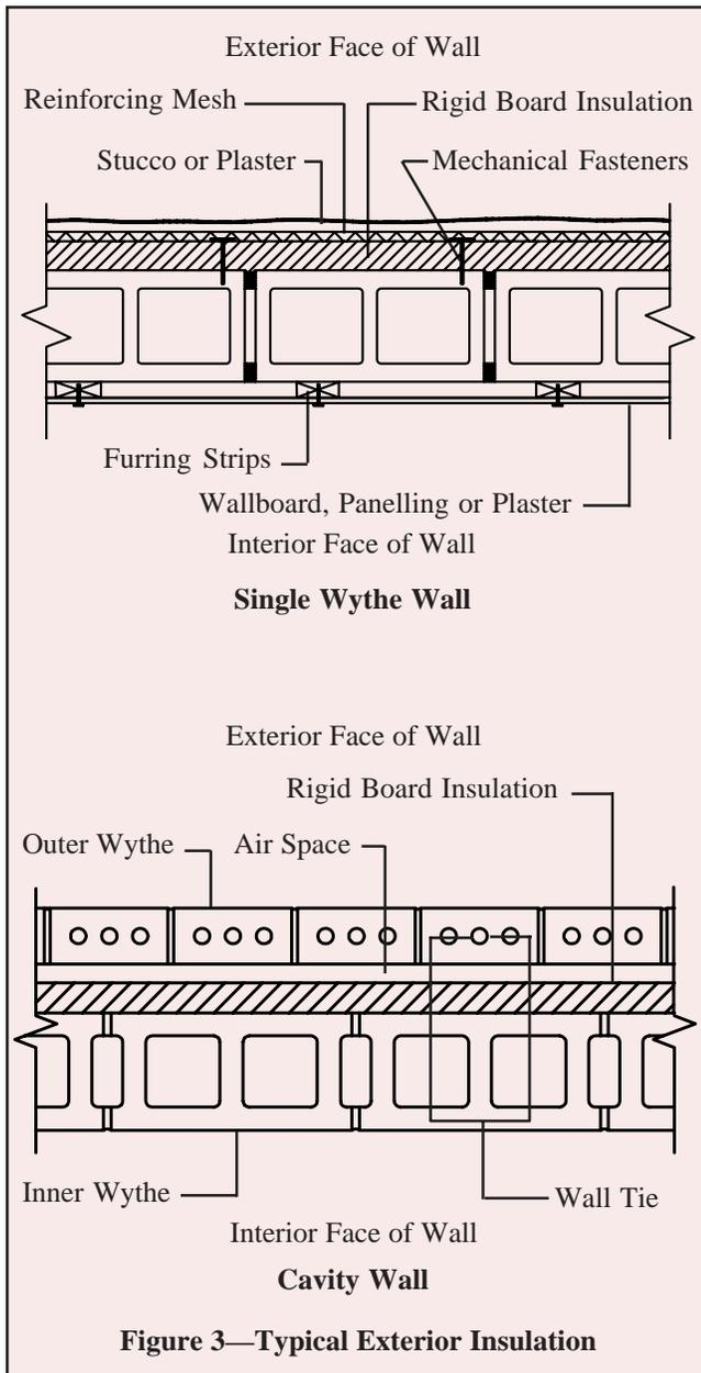
**Figure 3—Typical Exterior Insulation**
