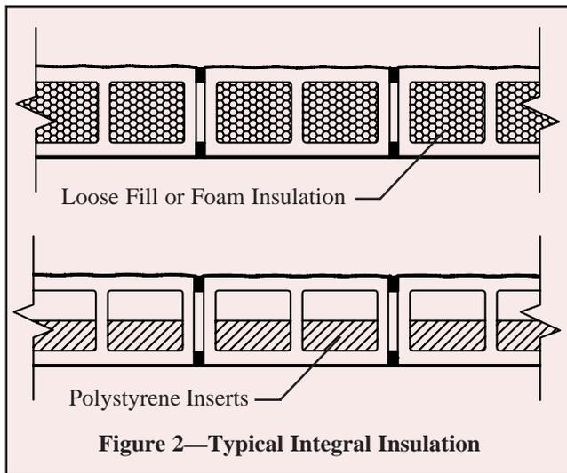
Figure 2—Typical Integral Insulation
