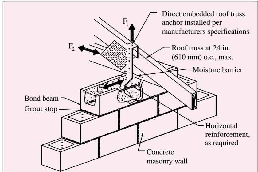
Note:  $F_1$ ,  $F_2$  and  $F_3$  are forces that must be accommodated in the design of the roof/wall connection.
