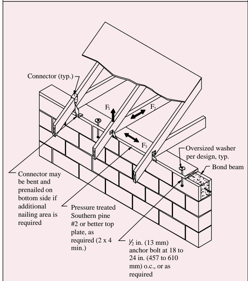
Note:  $F_1$ ,  $F_2$  and  $F_3$  are forces that must be accommodated in the design of the roof/wall connection.
