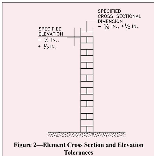
**Figure 2—Element Cross Section and Elevation Tolerances**
