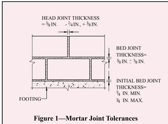
**Figure 1—Mortar Joint Tolerances**
