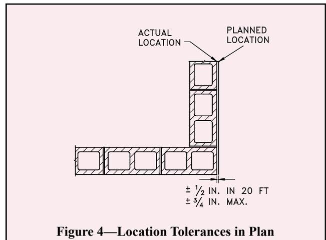
**Figure 4—Location Tolerances in Plan**
