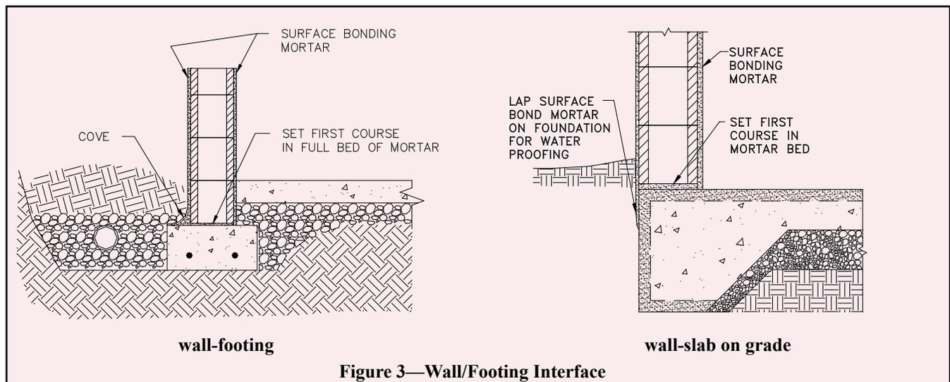
Figure 3—Wall/Footing Interface
