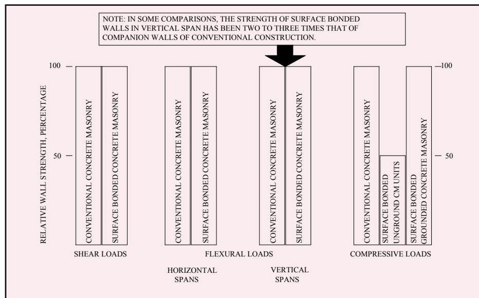
Figure 1 for ungrouted, unreinforced walls. Although national building codes, such as the *BOCA National Building Code* and the *Standard Building Code* (refs. 1, 3) do not specifically address reinforced or grouted surface bonded walls, manufacturers of surface bonding mortars may have code-approved criteria for their products.
