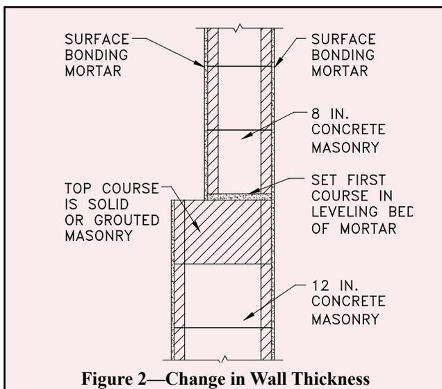
Figure 2—Change in Wall Thickness
