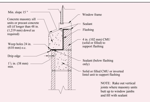
Figure 6—Flashing Single Wythe Walls at Sills
