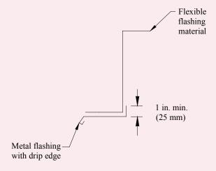
Figure 5—Two-Piece Flashing Detail
