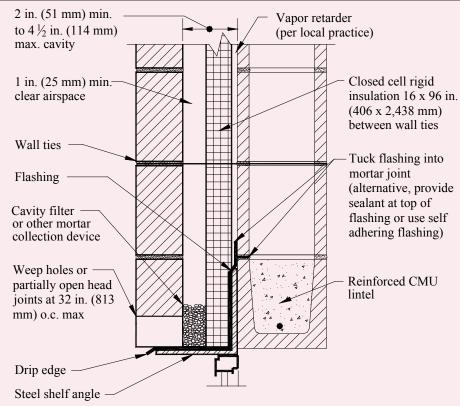
Figure 2—Flashing Cavity Walls at Bond Beam Locations
