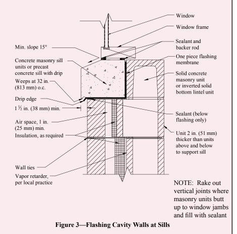
not taken, it is suggested that a wider airspace be utilized, i.e.  $1\frac{1}{2}$  to 2 in (38 to 51 mm). Also when using glazed masonry veneer, a 2 in. (51 mm) minimum airspace is recommended with air vents provided at the top and bottom of the wall because of the impermeable nature of the unit. Proprietary insulated drainage boards or mats are available that provide an unobstructed drainage path that eliminate the need for a clear airspace (ref. 4).
