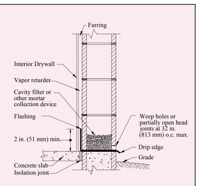
NOTE: The structural effect of throughwall flashing must be carefully evaluated.
