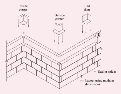
Figure 7—Prefabricated Flashing Boots
