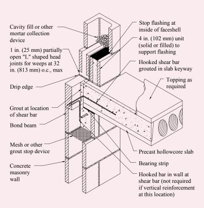
Figure 4—Flashing Single Wythe Walls
