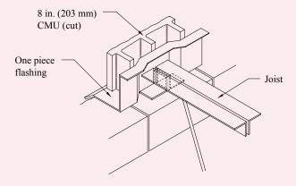
Figure 8a—Isometric of Flashing Around End of Joist (ref. 5)
