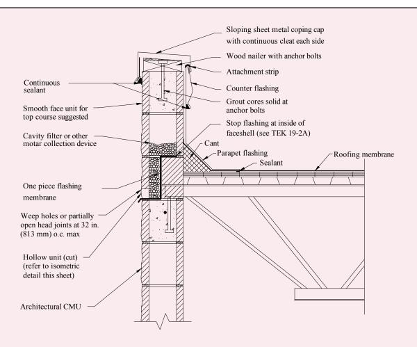
Figure 8—Flashing Single Wythe Walls at Roof/Parapet Intersection (ref. 5)
