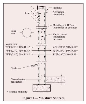
different temperatures, will move from the higher temperature to the lower. As air is cooled, it becomes more saturated and when it reaches a temperature called the dew point, the water vapor will condense into liquid form. See Figure 1.
