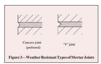
as they do not compact the mortar and/or create ledges that intercept water running down the face of the wall. Head and bed joints need to be the full thickness of the face shells for optimum watertightness. Head joints particularly are vulnerable to inadequate thickness (see Figure 4).
