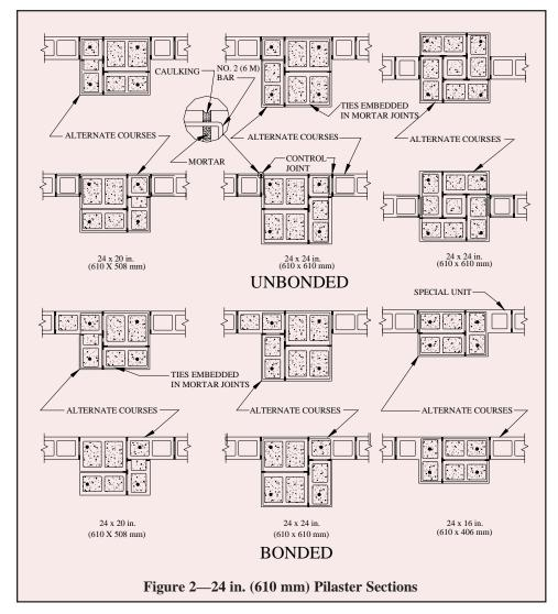
posed by beams or other framing members. When this occurs, pilasters are designed as columns and function as primarily as compression members. A chart for the selection of appropriate pilaster size and reinforcement for a variety of lateral loading conditions is presented in Table 1.
