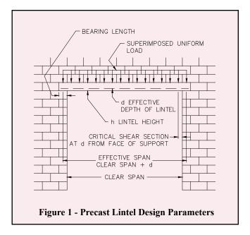
becoming factored loads. The lintel is then sized to provide sufficient design strength. Further information on determining design loads for lintels is included in *Allowable Stress Design of Concrete Masonry Lintels*, TEK 17-1A (ref. 3).
