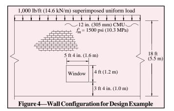
$M_{max} = 357 + 644 = 1,001 \text{ ft-lb} = 12,012 \text{ in-lb}(1.4 \text{ kN-m})$  $V_{max} = 251 + 339 = 590 \text{ lb}(2.6 \text{ kN})$
