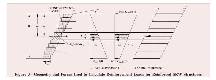
component of reinforcement load.
