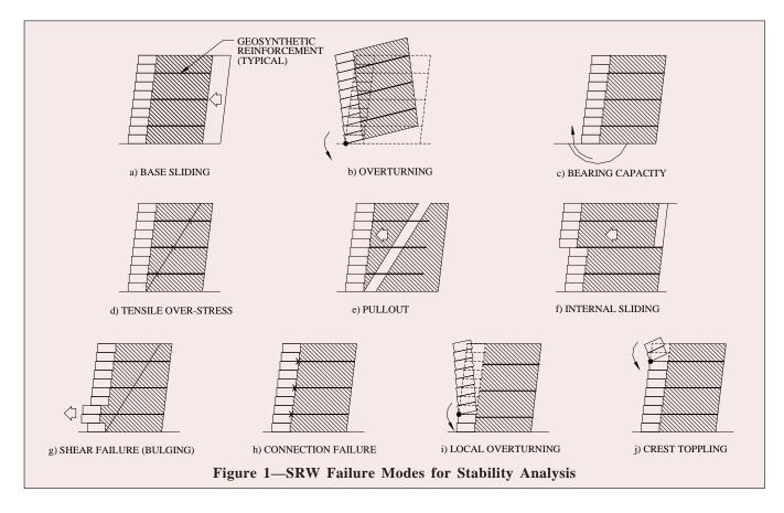
overturning about the toe, and foundation bearing capacity is similar to that used for conventional reinforced concrete masonry gravity structures.
