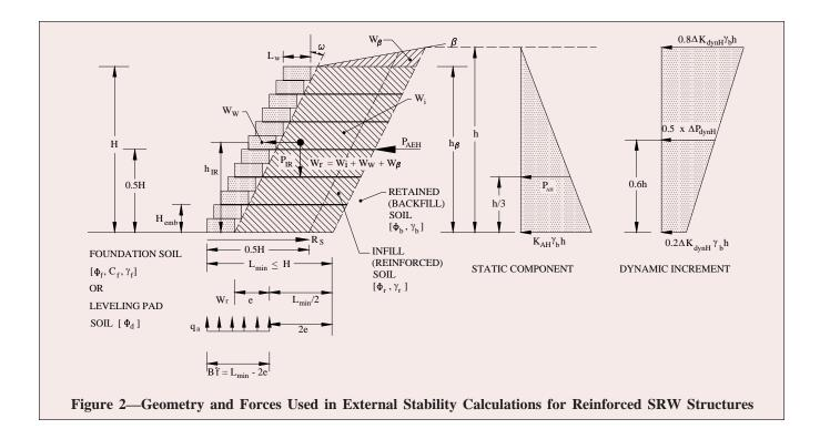
soils is not considered here. Separate calculations for foundation-induced deformations may be required by the designer. In addition, slope instability involving volumes of soil beyond and below the base of the facing column is not considered. Slope stability computer programs are available that can consider the effect of both the stabilizing influence of reinforcement layers and destabilizing influence of seismic-induced ground acceleration (ref. 2).
