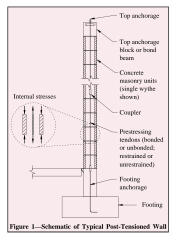
top and bottom of the masonry element (see Figure 1). Posttensioning is the primary method of prestressing, where the tendons are stressed after the masonry has been placed. This TEK focuses on the design of concrete masonry walls constructed with vertical post-tensioned tendons.
