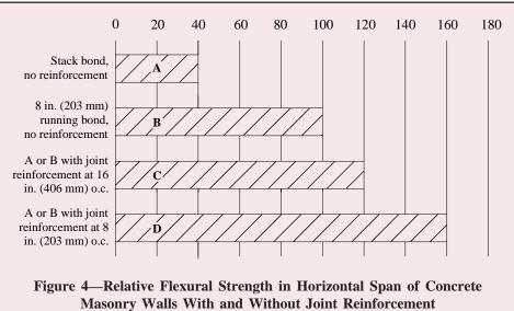
and details followed those specified in *Standard Methods of Conducting Strength Tests of Panels for Building Construction*, ASTM E 72 (ref. 3)
