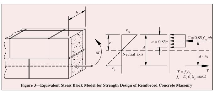
balanced strain conditions,  $\rho_{bal}$  (ref. 7). Balanced conditions occur when reinforcement reaches its specified yield strength at the same time that masonry reaches its maximum usable compressive strain of 0.003. This limit on reinforcement ensures the steel yields at strength level loads.
