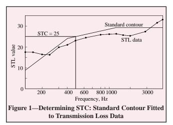
Although STC is a convenient index of transmission loss, it may be necessary in some cases to study the sound transmission loss data at specific frequencies, such as when the main noise source is of one known frequency. In this case, the STL value at the frequency of interest is checked to ensure there is not a "hole," or low STL value, at that particular frequency.
