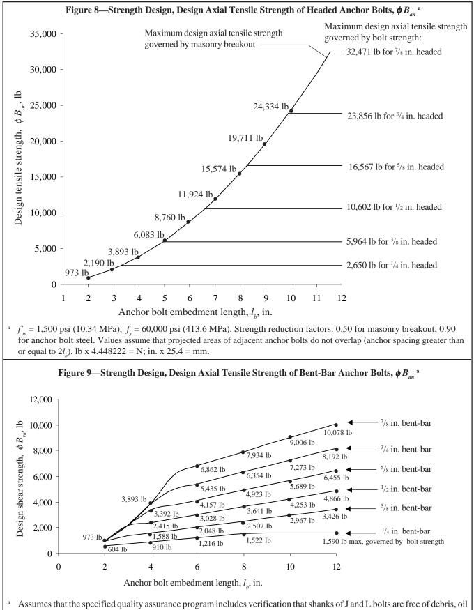
and grease when installed.  $f'_m = 1,500 \text{ psi} (10.34 \text{ MPa}), e_b = 2d_b, f_y = 36,000 \text{ psi} (248.2 \text{ MPa}).$  Strength reduction factors: 0.50 for masonry breakout; 0.90 for anchor bolt steel; 0.65 for anchor pullout. Values assume that projected areas of adjacent anchor bolts do not overlap (anchor spacing greater than or equal to  $2l_b$ ). Ib x 4.448222 = N; in. x 25.4 = mm.
