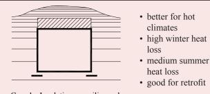
Case 1 - Insulation on ceiling only Seasonal Performance Heating: Poor Cooling: Good
