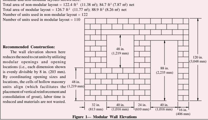
of concrete masonry units are typically  ${}^{3}/{8}$  in. (9.5 mm) less than nominal dimensions, so that the 4 or 8-in. (102 or 203 mm) module is maintained with  ${}^{3}/{8}$  in. (9.5 mm) mortar joints. Where mortar joint thicknesses differ from  ${}^{3}/{8}$  in. (9.5 mm) (as may be specified for aesthetic purposes or with brick construction), special consideration is required to maintain modular design. Figure 3 illustrates this concept.
