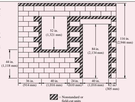
In this example, it is obvious the aesthetic impact non-modular layouts have on the final appearance of a structure. Not so obvious is the additional cost of construction. To further illustrate this concept, consider the following comparison of the modular and non-modular layouts shown here:
