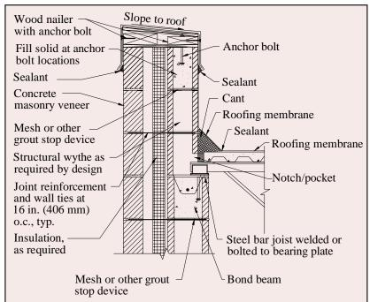
Notes: Structural wythe of parapet must be a minimum of 8 in. (203 mm) thick when empirical design is used (ref. 1). Rational design may allow a thinner wythe. Extending insulation up the full height of the parapet helps prevent thermal losses through the parapet.
